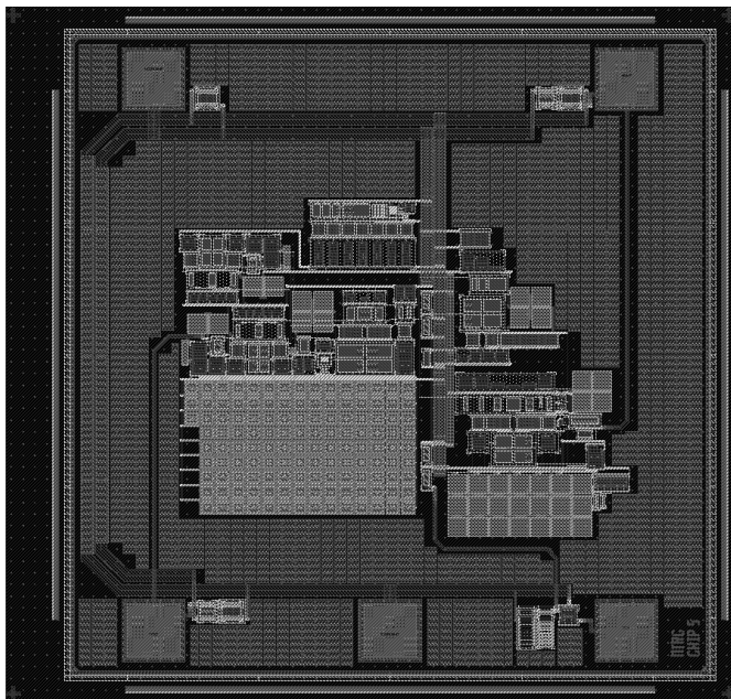
Figure 7. Chip layout for the pre-amplifier and regulator (for AMP2)
